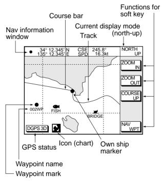
Figure 3-1 Plotter display, north-up mode
